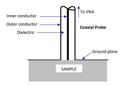
Figure 2: Coaxial Probe
